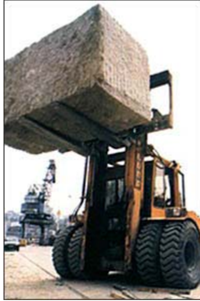
Figure 19. Use extra caution when carrying loads that approach a vehicle's maximum design limits.
