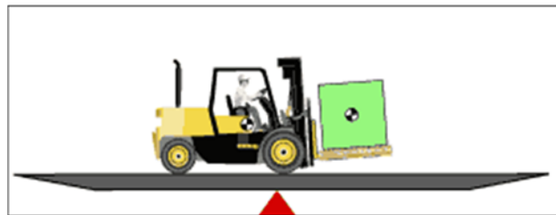
Figure 18. The forklift teeters and finds its balance point. As the load is added to the seesaw, the moment is increased on the right side. The loaded forklift reverses and finds a new balance point at its combined center of gravity.
