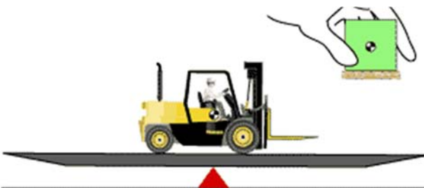
Figure 12. Notice the center of gravity of the load and truck system shift forward toward the front wheels as the load is engaged.
