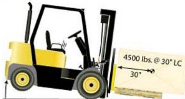
Figure 7. Improperly distributed loads may tip the forklift if the maximum load moment is exceeded.
